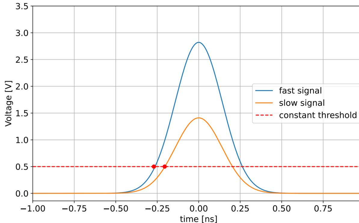
**Example of the time walk effect.** Although both signals reach their maximum at the same time, the threshold-crossing time is different.
