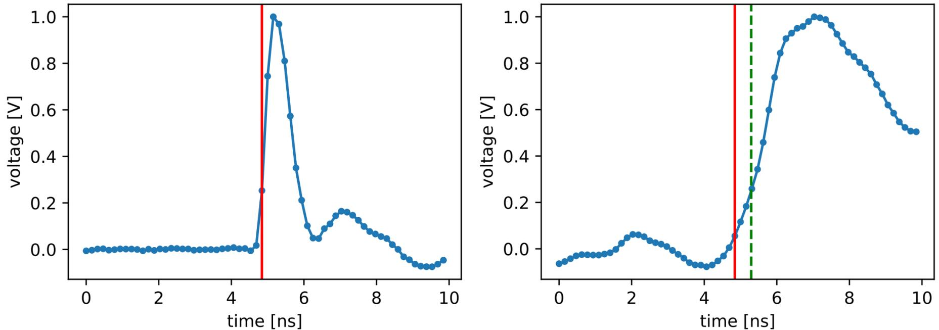
**Dataset example.** Left: an MCP signal with marked ground-truth timestamp. Right: a signal from a diamond detector; red: the ground-truth timestamp (includes the  $t_0$  shift of both signals), green: the CFD timestamps computed on the diamond detector time series (used to compare the neural networks with CFD).
