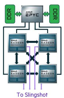
2560 nodes with 4 x MI250X + 1 x AMD Trento processor, 512 GB host memory and 512 GB device memory (HBM2) 4 x 200 Gbit/s NIC Infinity Fabric
