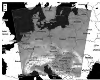
Fig. 1. Extent and topography of the WRF domain for the parent domain (5 km) and location of two subdomains (1 km and 200 m) marked with rectangles.
