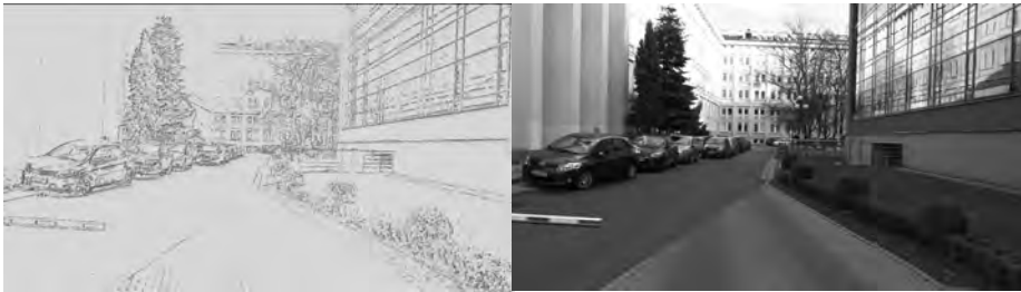
Fig. 1. Comparison of a frame from a classic camera and an event frame aggregated over 20 ms.
